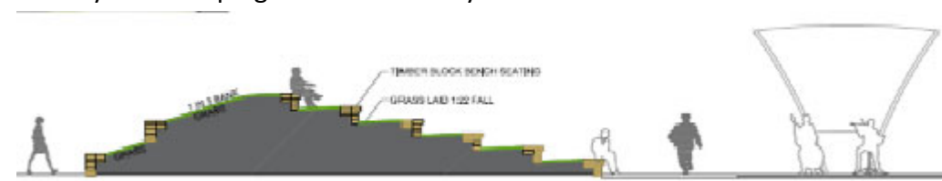
Section through proposed Amphitheatre and stage canopy
